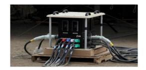
Description: The Mobile Power Distribution Box is a 800 Amp, 3 Phase, 4 Pole, 5 Wire, 120/208Y VAC, (2) sets of (5) 16 Series Cam-type color-coded panel mount inlets to (4) 100 Amp MIL-DTL-22992 receptacles, (10) 60 Amp MIL-DTL-22992 receptacles, and (1) NEMA 5-20, 20 Amp GFCI duplex receptacle, Rubber Enclosure with Ridged HDPE Top and Bottom - Weather Resistant.
